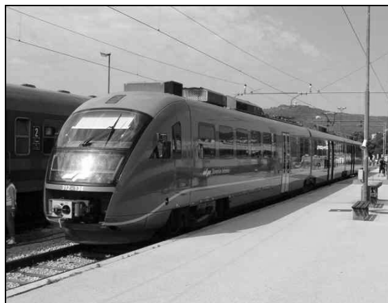
Figure 5. The Siemens three-part motor – coach train Series 312, rated output 1 MW
